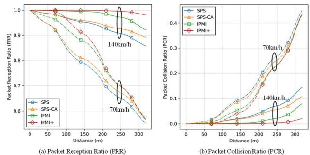
**FIGURE 7. Reliability in the 70 or 140 km/h scenarios (freeway model): (a) Packet reception ratio (PRR), (b) Packet collision ratio (PCR).**
