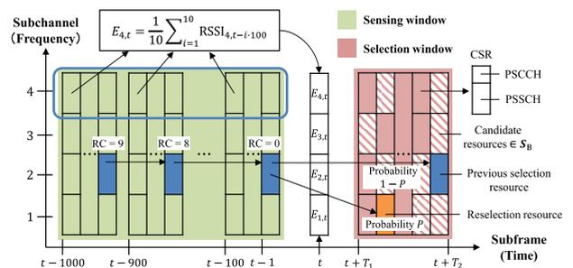
FIGURE 1. Resource reselection with the SPS algorithm (RR1 = 100ms).
