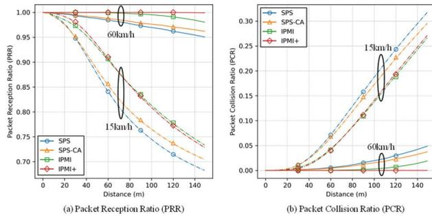
**FIGURE 6. Reliability in the 15 or 60 km/h scenarios (urban model): (a) Packet reception ratio (PRR), (b) Packet collision ratio (PCR).**
