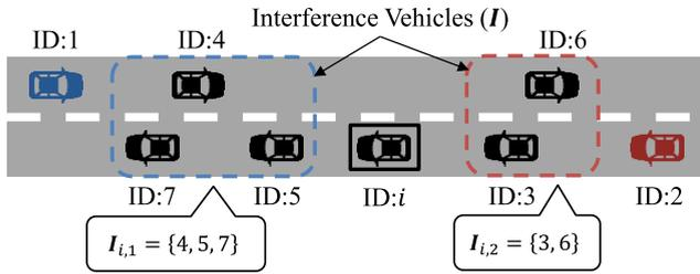
FIGURE 2. Set of interference vehicles.
